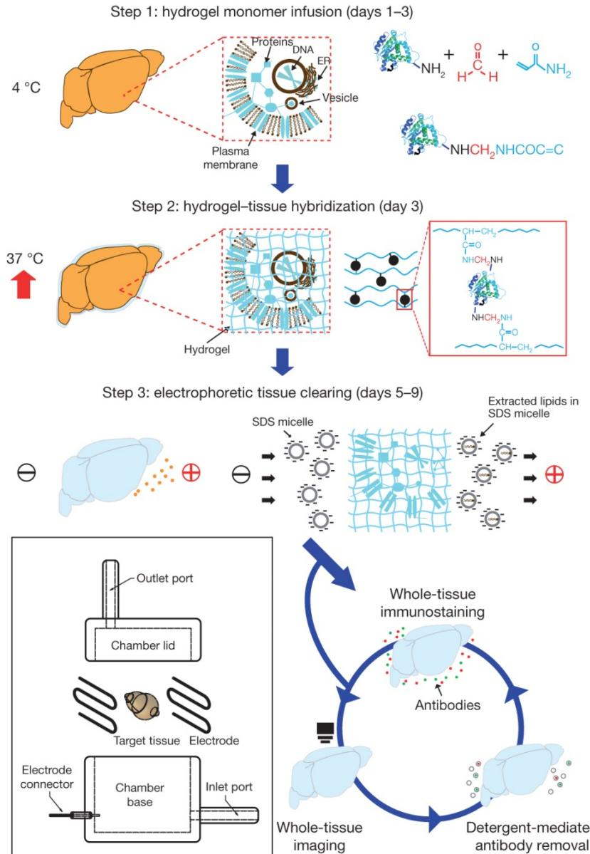
Tissue is crosslinked with formaldehyde (red) in the presence of hydrogel monomers (blue), covalently linking tissue elements to monomers that are then polymerized into a hydrogel mesh (followed by a day-4 wash step; Methods). Electric fields applied across the sample in ionic detergent actively transport micelles into, and lipids out of, the tissue, leaving fine-structure and crosslinked biomolecules in place. The ETC chamber is depicted in the boxed region
