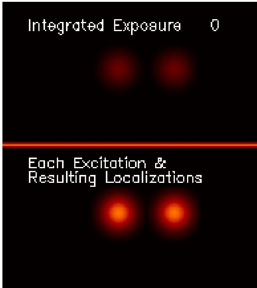
A small fraction of a sample's fluorescent proteins are put into an "on" state, where they glow red when illuminated with yellow light. At the highest optical magnification each molecule looks like a fuzzy ball about 250 nm in diameter. However, the center where the fluorescent label is located can be determined to a fraction of that size.
