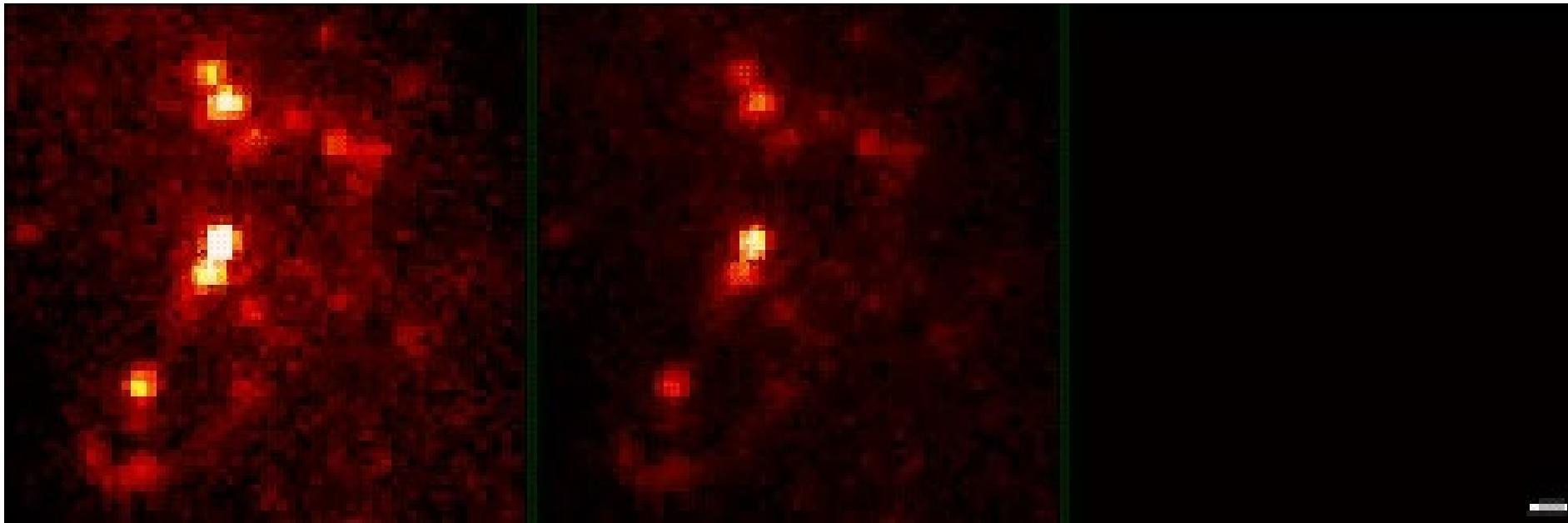
Gradual assembly of a photoactivated localization microscope (PALM) image (right) from the center coordinates of the images of many single molecules (flashing spots at left), activated and localized one-at-a-time. If the images are summed without localization, the conventional optical image is eventually recovered (center).
